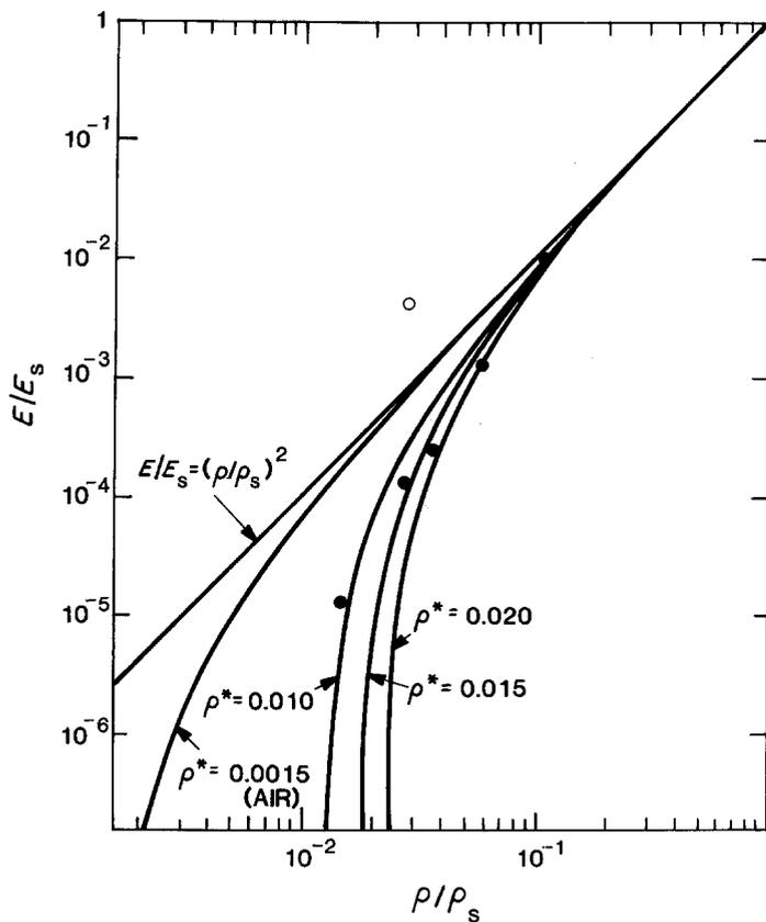
Figure 6 Influence of noncontributing material on the magnitude of the reduced elastic modulus at reduced material density. (Data at 0.25 mm penetration. Curves from Equation 3 or 5.) (○) PS ( $E_s = 1400$  MPa), (●) PMP-A ( $E_s = 900$  MPa).
