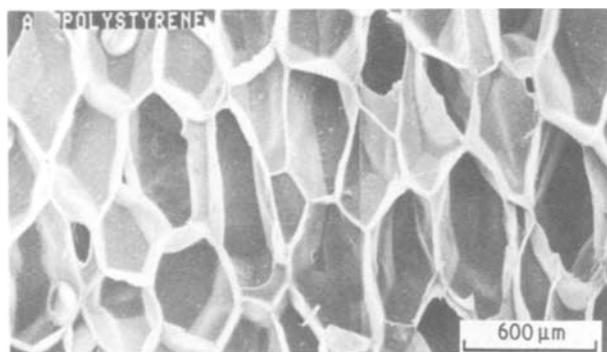
Figure 5 SEM of polystyrene foam board ( $\rho = 0.031 \text{ g cm}^{-3}$ ).
