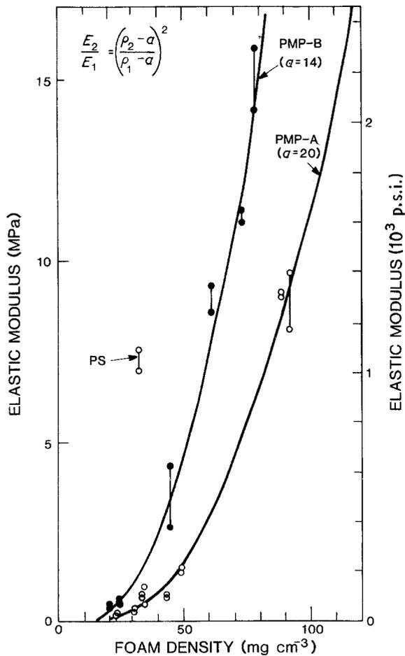
Figure 1 Elastic moduli of low-density foams. (Data at 0.76 mm penetration. Curves are based on Equation 2.)
