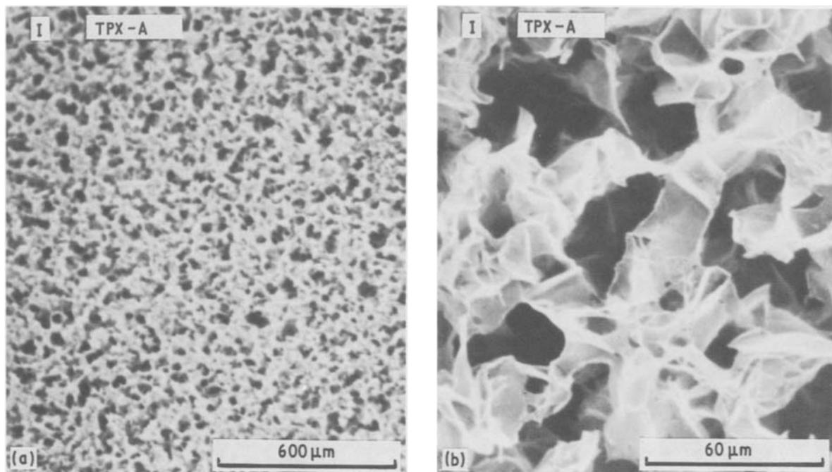
Figure 4 SEM of PMP foam prepared by Method B ( $\rho = 0.020 \text{ g cm}^{-3}$ ).
