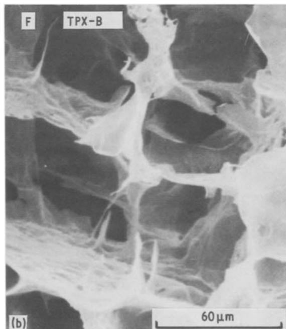
Figure 3 SEM of PMP foam prepared by Method A ( $\rho = 0.034 \text{ g cm}^{-3}$ ).
